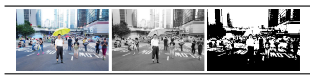
Figure A.8: Left, the original image. Center, the image in grayscale. Right, the image thresholded according to Otsu's method. All three images are filtered.
