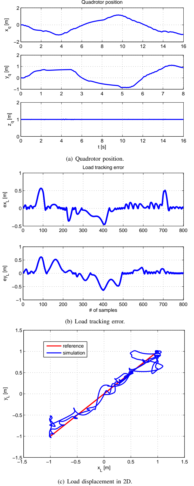
Fig. 4. Simulation results for online LSPI used for suspended load tracking the straight line.
