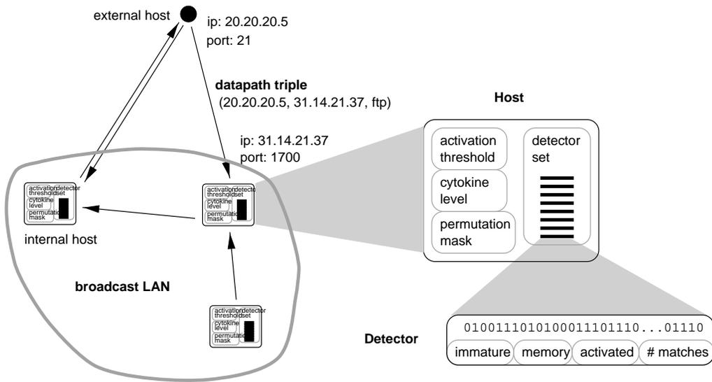
Figure 1: Architecture of Artificial Immune System.
