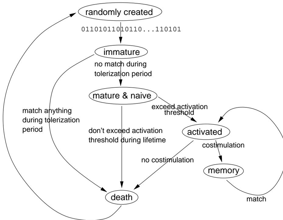
Figure 2: The Lifecycle of a Detector.
