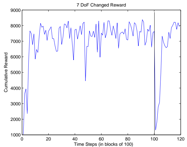
Fig. 4: Cumulative reward for running in simulation and then transferring the task to hardware. The transfer occurs at 100 blocks.
