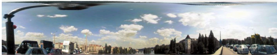
Figure 3: 360° panorama computed by geometric correction of image of cone shaped mirror.
