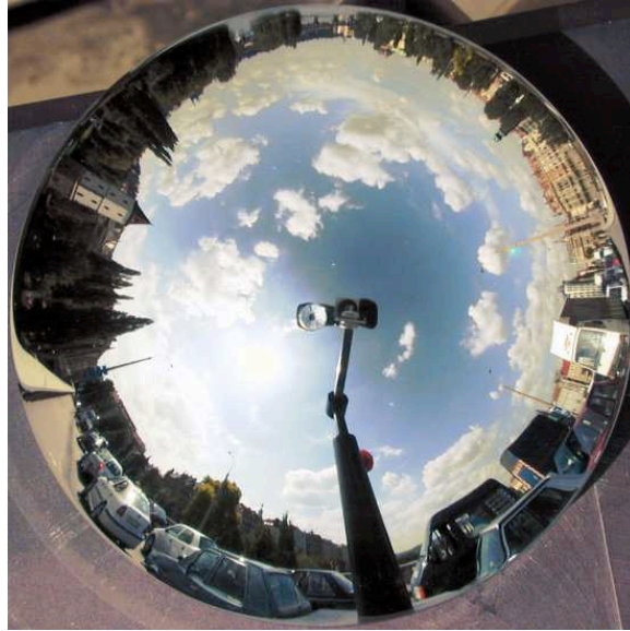
Figure 2: An image take by a camera pointed at a cone shaped mirror.
