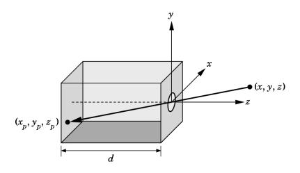
Use trigonometry to find projection of point at (x,y,z)
