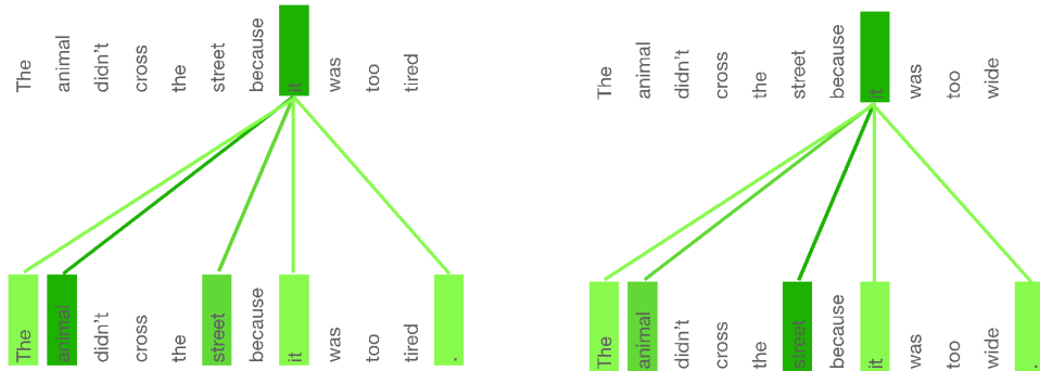
Fig. 14. Attention: finding the relevant tokens supporting use of the pronoun “it” in two different but syntactically related sentences. Figure adapted from [2].
