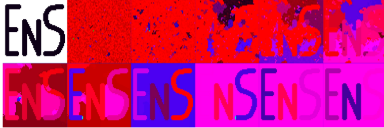
Figure 4: Time series evolution of spiking neurons for image segmentation, from [18]. Areas of similar color are similar activation level
