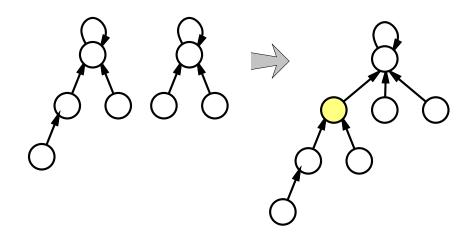
Merging two sets stored as trees. Arrows point to parents. The shaded node has a new parent.
