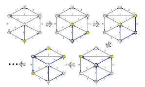
Four phases of Dijkstra's algorithm run on a graph with no negative edges. At each phase, the shaded vertices are in the heap, and the bold vertex has just been scanned.
