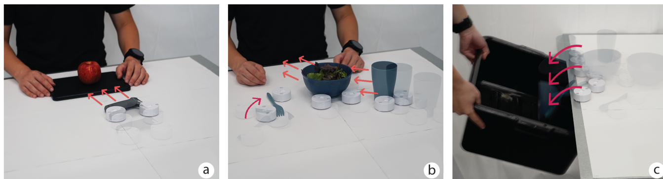
Figure 12: Cooking and Dining Application (a) Robots bring a far-away peeler to the user when he needs to peel an apple. (b) The system sets the table for the user by bringing and arranging the tableware in a desired configuration. (c) After dining, robots push the dirty dishes to the edge of the table so they fall into the dish-cleaning bin.
